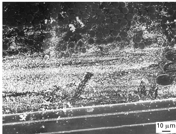
Figure 1 SEM micrographs shows the distribution of particles (appears in white colour) inside the composites.
